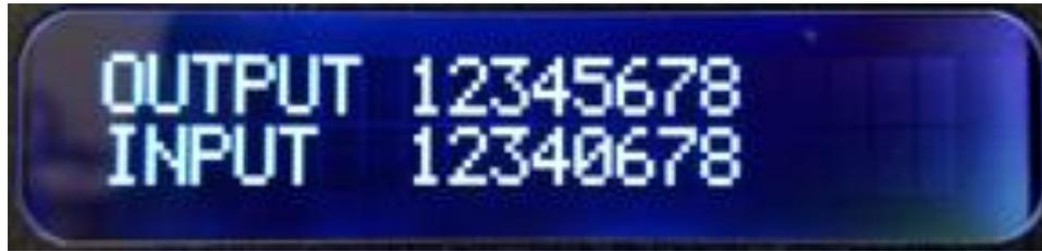
The LCD will reflect what Output is routed to which input when in an idle state.
